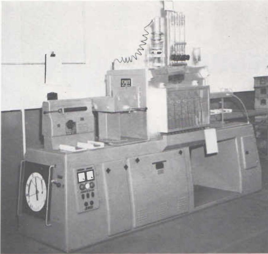
Continuous kiln for firing small ferrite products.
