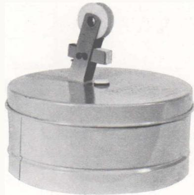
(b) Lid for use with dynamic or static tensioning.
