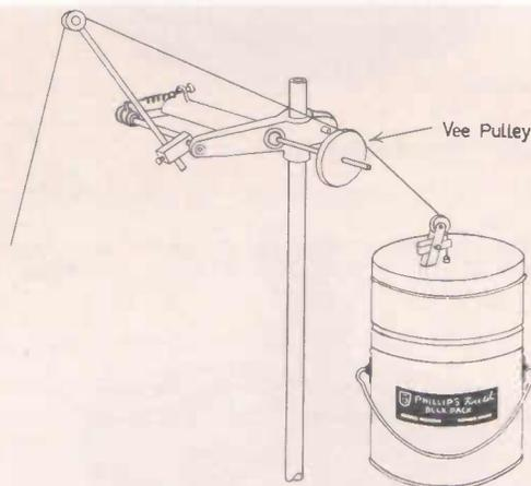
Fig. 3. Details of tensioning mechanism in Fig. 2 above.
