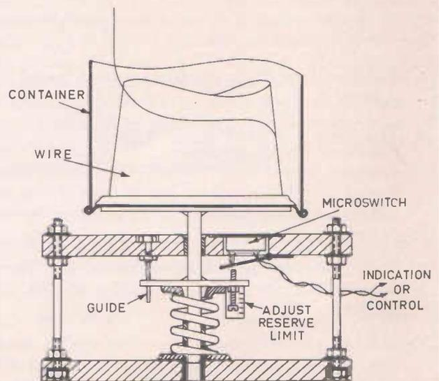
Fig. 5. Suggested actuating device to provide winding safeguards.
