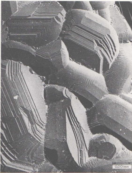
Surface of Ferroxdure ferrite showing crystal structure. Magnification 10,000 diameters.
