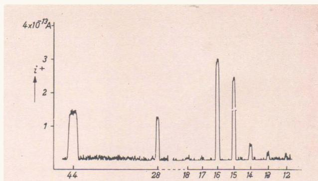
Fig. 2. Mass spectrogram obtained in studying the effectiveness of a barium getter.
