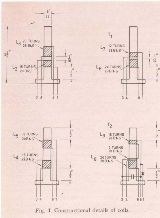
Fig. 4. Constructional details of coils.
