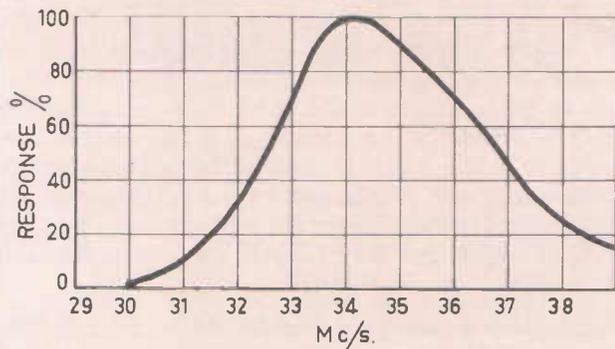
DETECTOR BANDPASS TRANSFORMER  $T_2$
