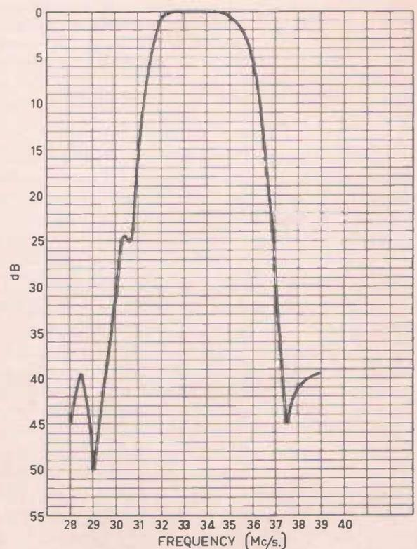
Fig. 3. Overall IF amplifier response for  $-1\text{ V DC}$  at detector and  $-5.0\text{ V}$  bias.
