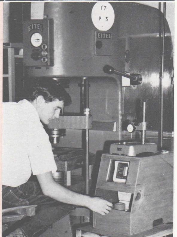
Operator checking weight of ferrite rings after pressing.
