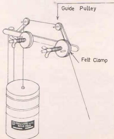
Fig. 4. Tensioning mechanism of static spool machine used with Bulk Pack.
