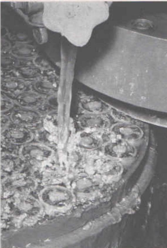
Surface grinding of ferrite half-cups.
