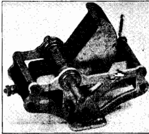
Typical of the condensers used in the late '20's is this "Pilot" type, with specially-shaped rotor plates. This condenser also has 23 plates in all and a capacitance of .0005 mfd.
