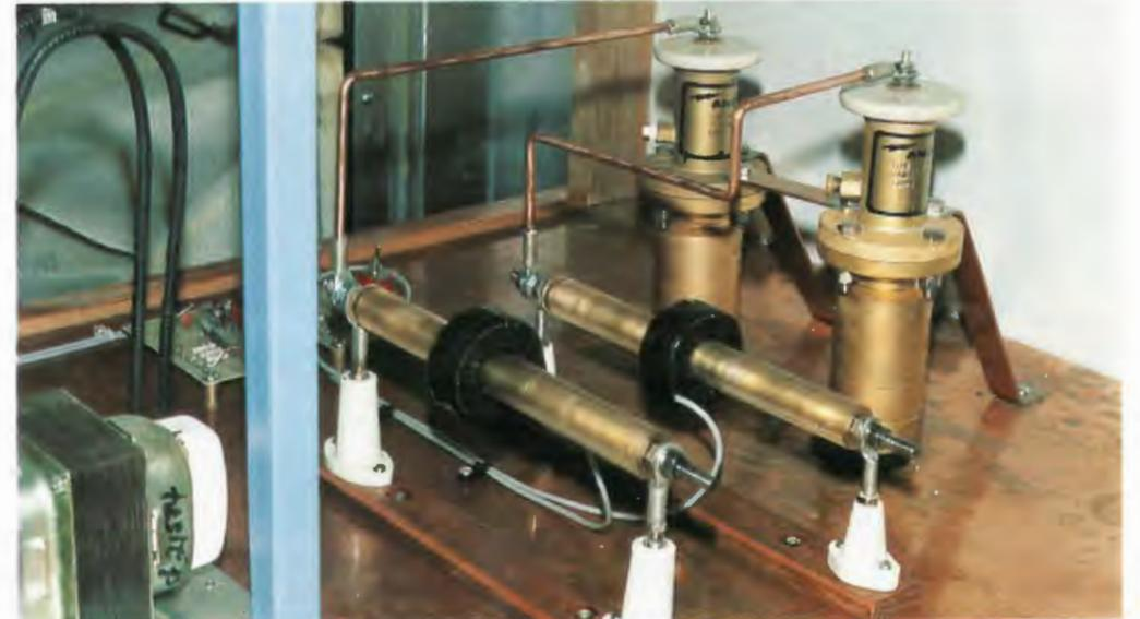
Cable terminations and line current transformers - 4CH.
