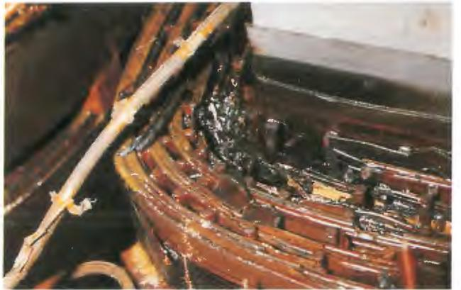
*Damage to secondary winding.*
