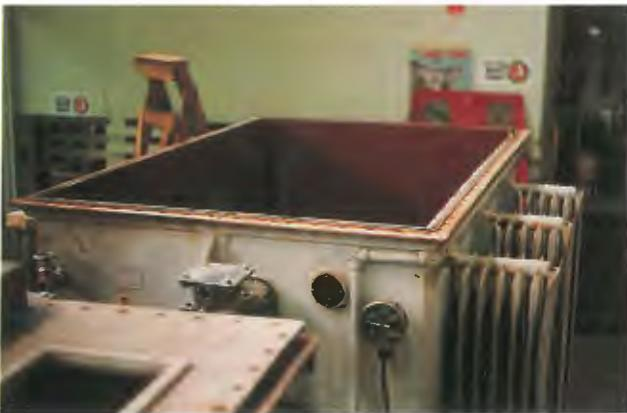
*Transformer tank with core removed.*
