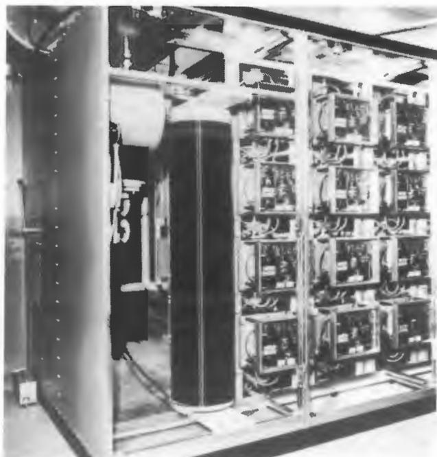
*Switching module showing some of the water cooled switching elements.*
