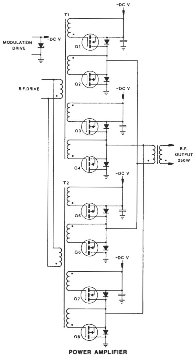
The power amplifier stage consists of eight 1.25 kW power blocks that combine in the output transformer to give the total 10kW output power. Each power block has three pairs of 250 W power amplifier modules, a modulator module and a rectifier/regulator module.
