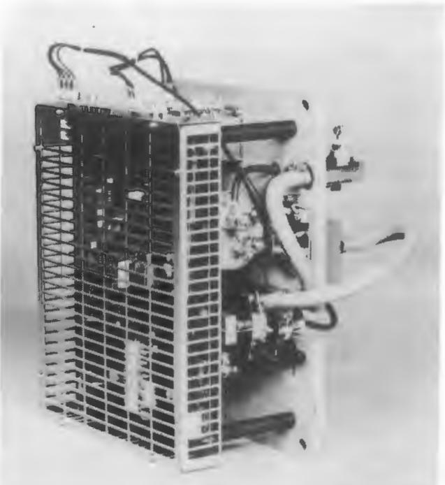
*Partial front view PSM amplifier showing pulse frequency filter and some switching stages.*
