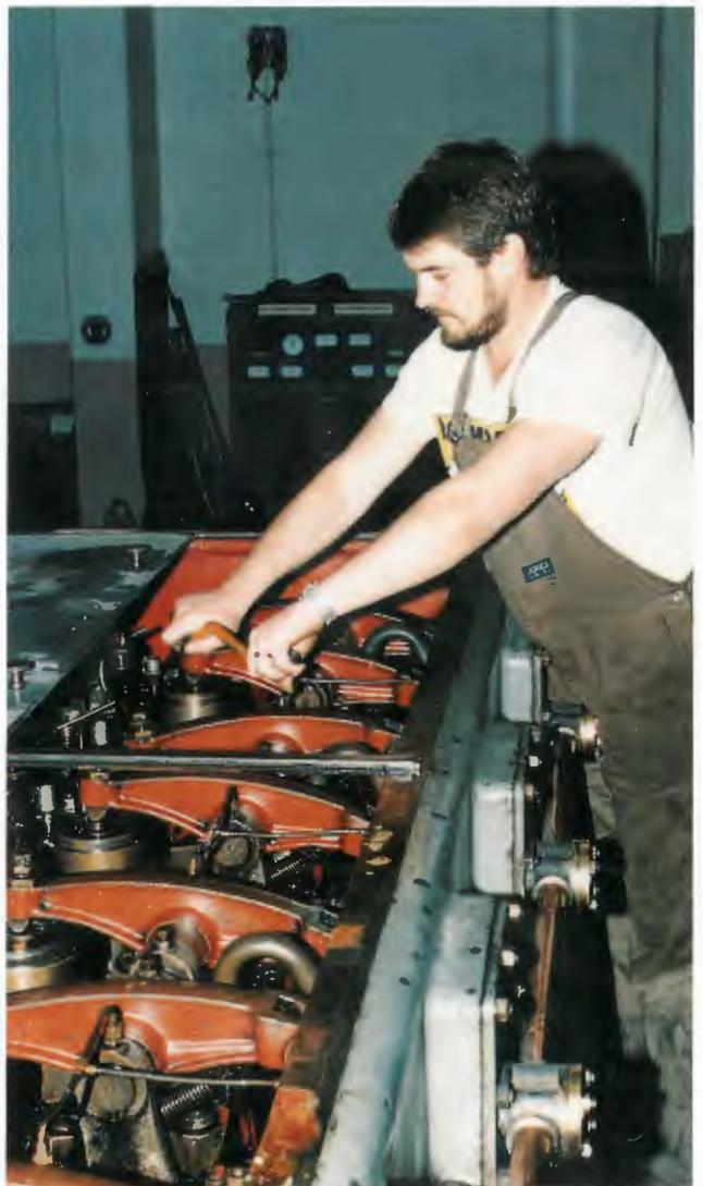
*Diesel Mechanic Steve Nankivell adjusting tappets on one of the Crossley 800 HP engines*
