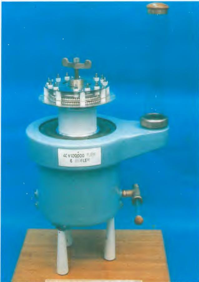
*Tube 4CV 100000 and boiler as used in power amplifier and modulator stages.*
