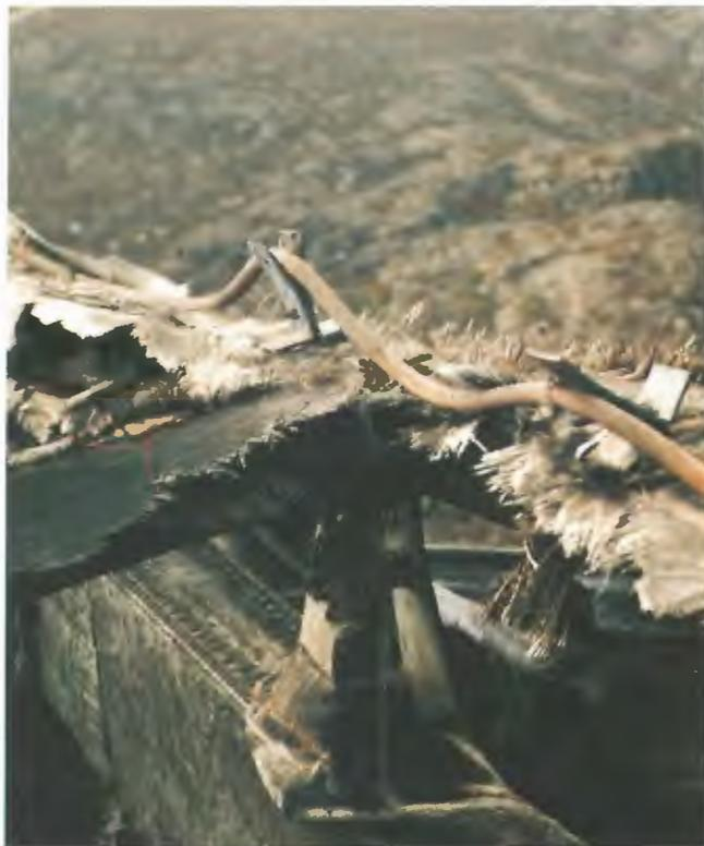
*Damaged fibreglass on radome top.*
