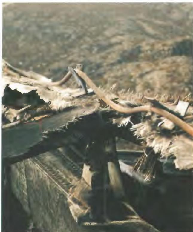
*Damaged fibreglass on radome top.*
