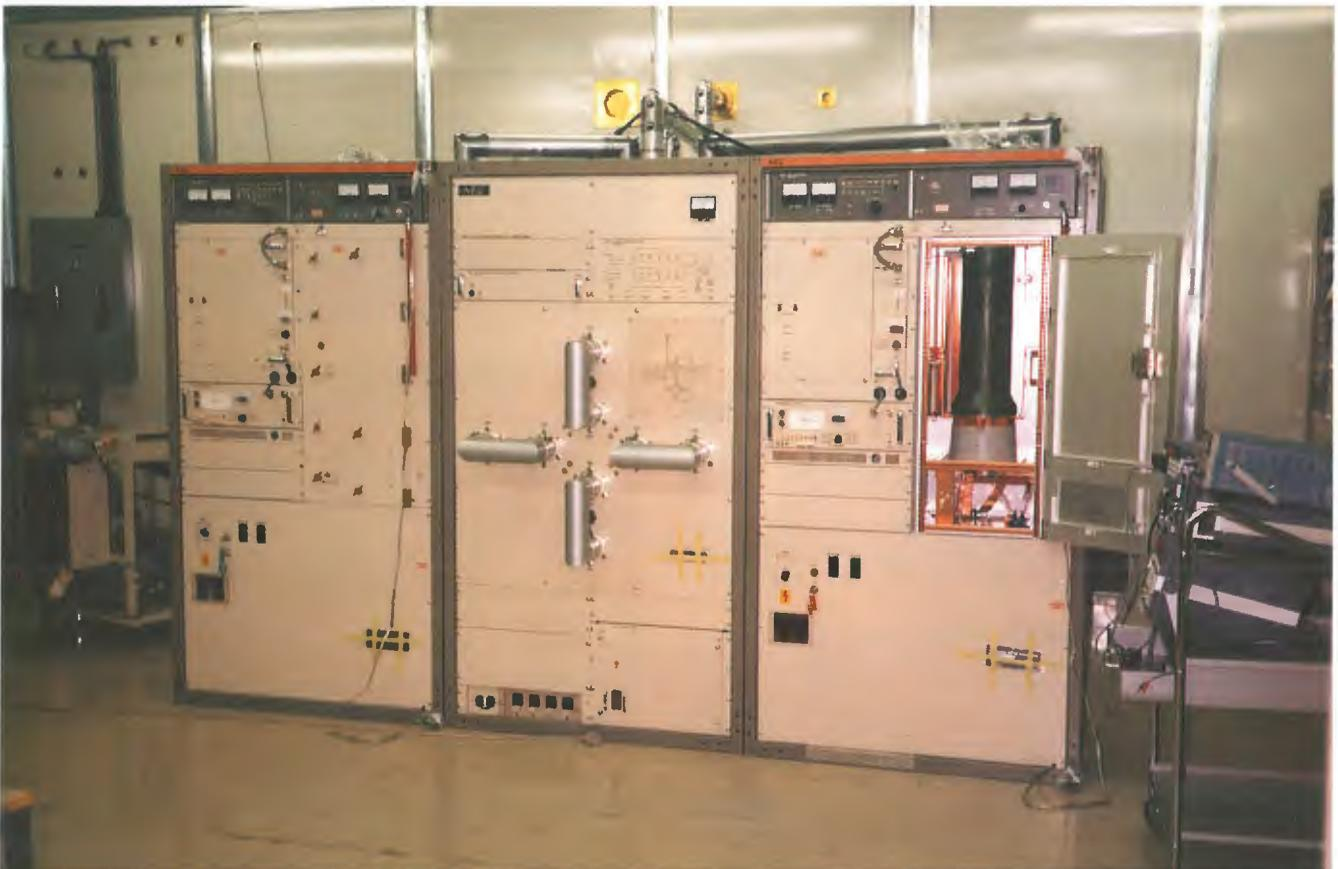
*Dual 10 kW FM transmitter in screened test room.*
