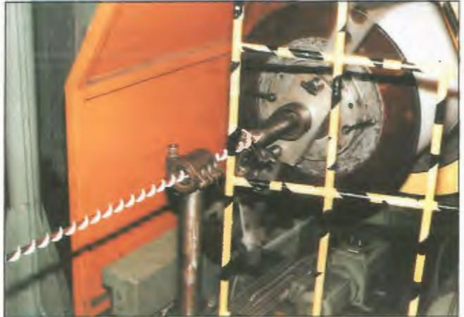
*Application of helix to centre conductor of FLEXWELL HF 7/8 inch Cu2Y cable.*
