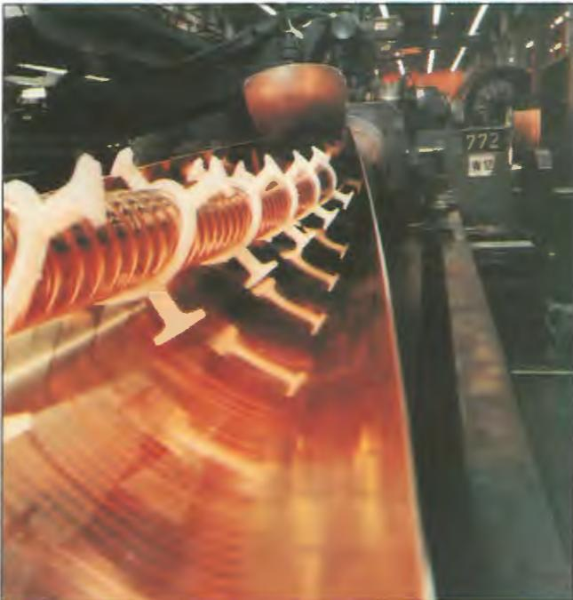
*Feeding and forming of outer conductor of large size cable.*
