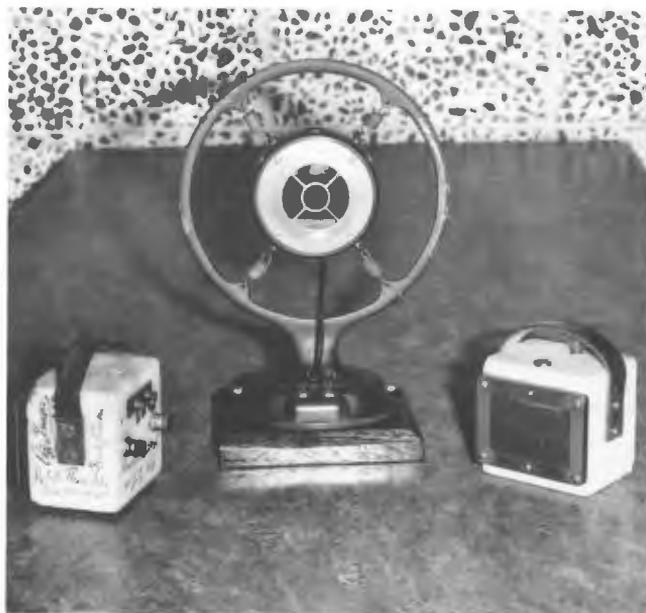
*Early 4QG carbon microphones. Locally made Reisz types and double button carbon type (centre).*
