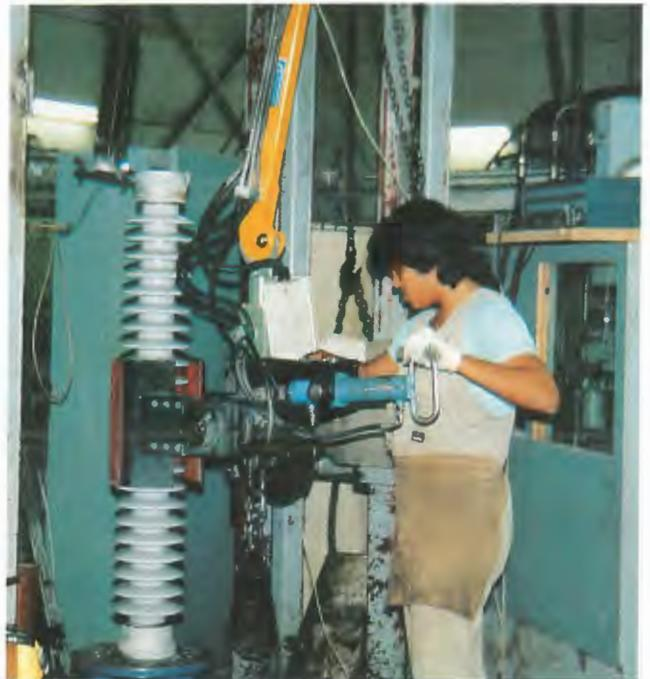
*Preparing an insulator for mechanical tests.*
