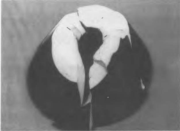
*Insulator damage caused by lightning.*
