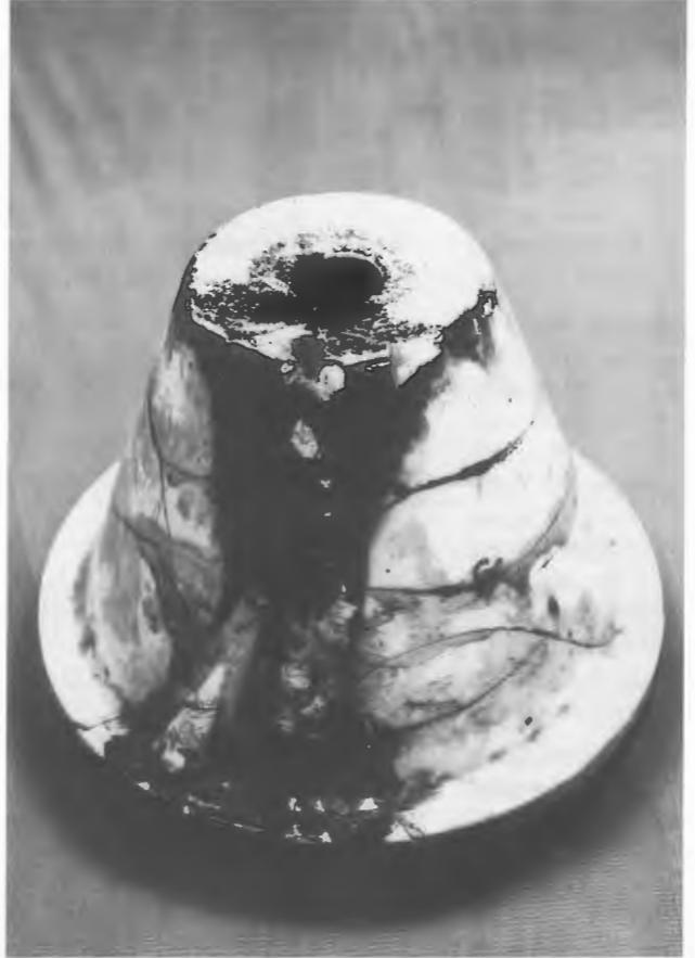
*Insulator damage caused by RF arc.*
