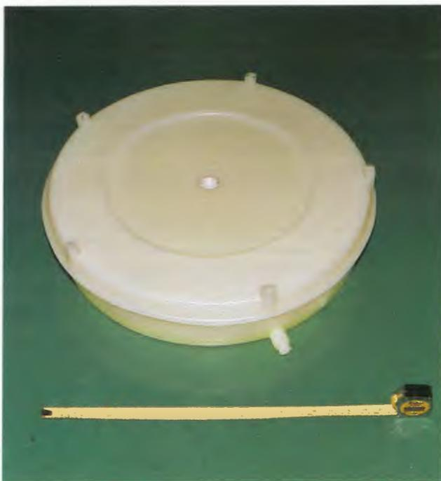
*Typical sealed sloshing damper container.*
