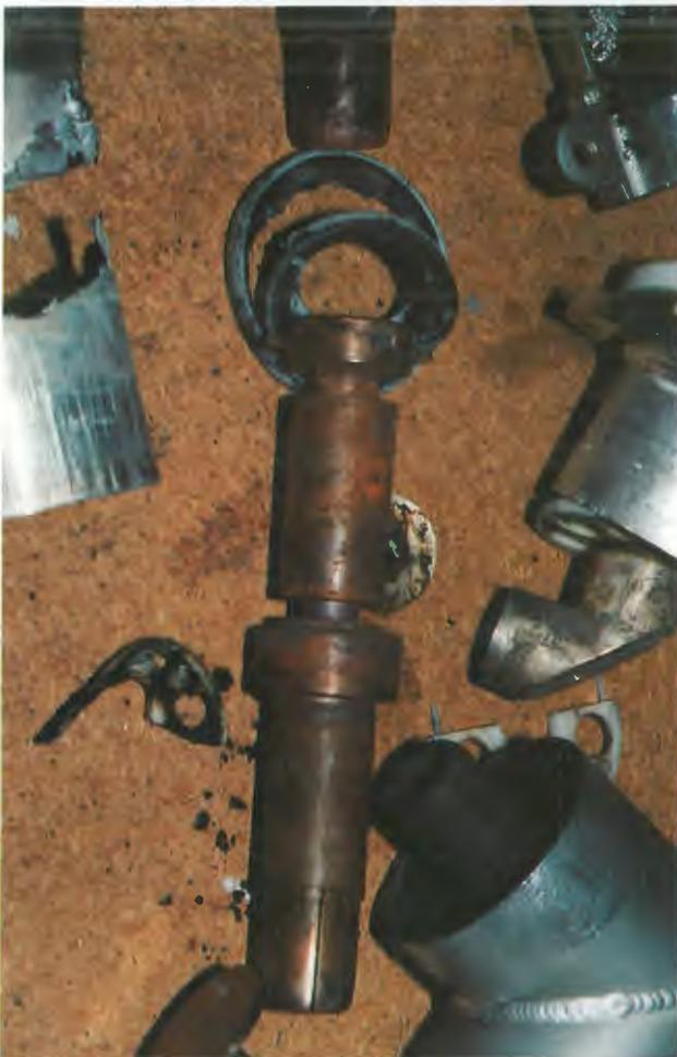
*Damaged components. Note centre portion of boot missing.*
