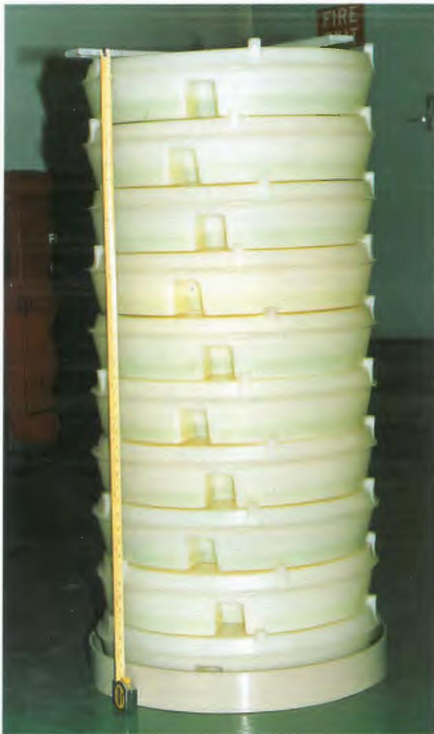
*Stack of 10 sloshing containers. Eight stacks were installed within Mt Wellington tower.*
