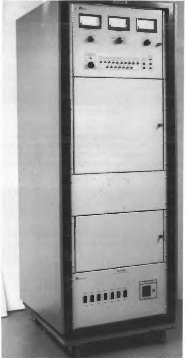
The 7kW AMFET FM7 solid state transmitter.
