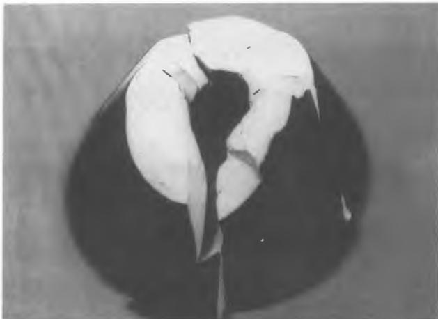
*Insulator damage caused by lightning.*
