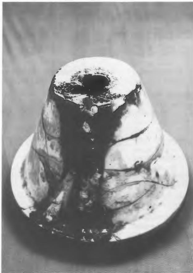
*Insulator damage caused by RF arc.*
