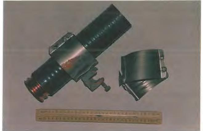
*Wind-induced vibration has caused fatigue failure of stainless steel cable clamp.*
