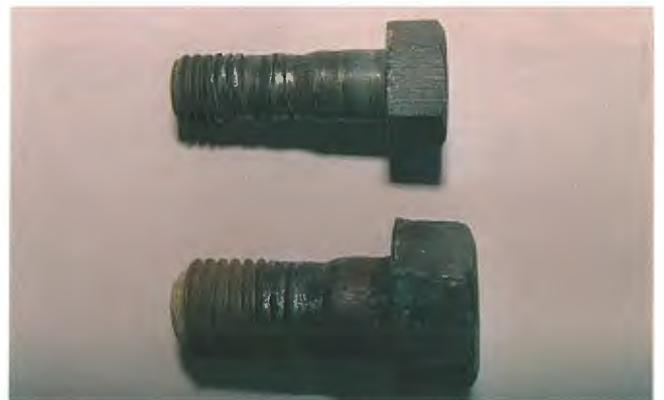
*Wind-induced vibration of structure caused hammering of connection bolts.*
