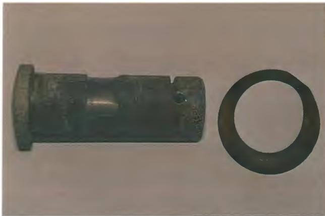
*Vibration has caused washer to cut into pin. Note elongated hole in washer and wear on pin.*
