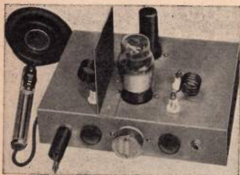
Figure 5. Simple One-Tube (R.F.) 5-Meter Transmitter
