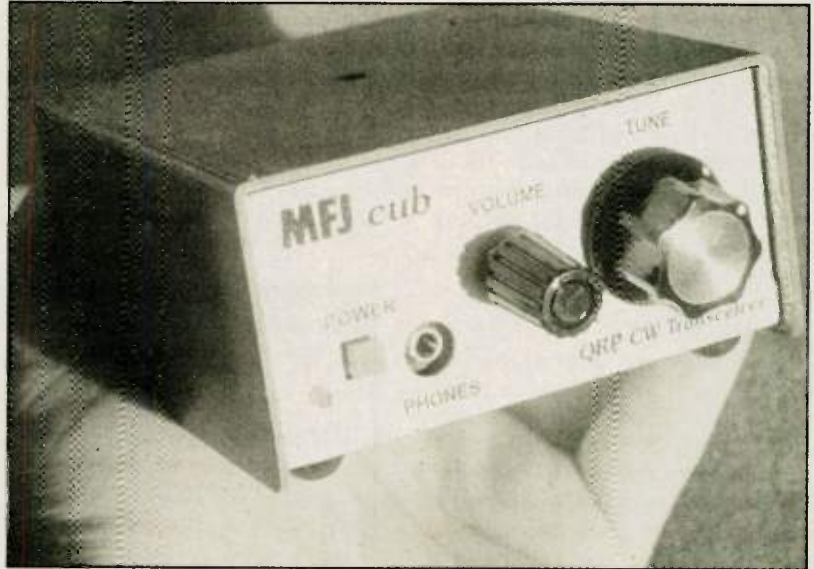
MFJ Enterprise's easy-to-build "Cub" QRP transceiver kit combines both surface mount and hole-through technologies.
