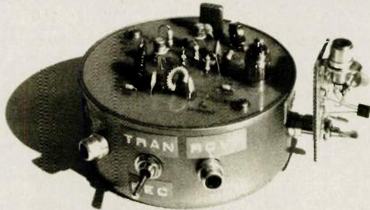
The Plus 1 PC board strikes a vertical pose after being plugged-in to the TT-2's 12 volt jack. A shorted phono plug is placed in the rig's original key jack atop the TT-2's PC board.
