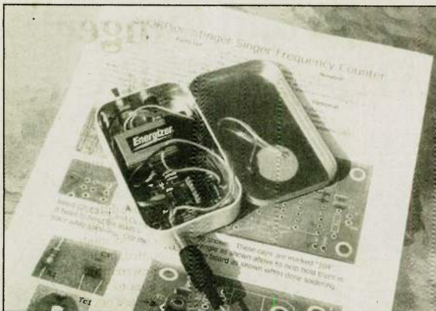
The AZ ScQRPion Stinger Singer frequency counter kit is designed for use in a classic Altoids-style light metal chassis.
