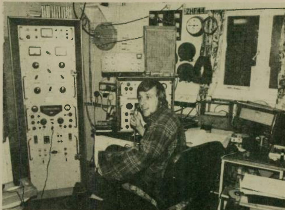
VP8NP/Ian Bateman (G3ZKH) opr on barren GALINDEZ ISL. ANTARCTIC 2 yr. Scientific EXPEDITION 65S/64W making IONOSONDE readings. Operates "Between Tests", on 160 meters!! 1.804 and 1.827 MHz, giving many this extremely rare 160 country, including W1BB's 117th. Uses balloon and dipole ants w/RA17 rig. Is well known member famous "White Rose" radio club. Cheers and Congratulations, Ian - VFB!! (QSL via G4BNH/Frank, who is doing VFB "Liaison" job!!)
