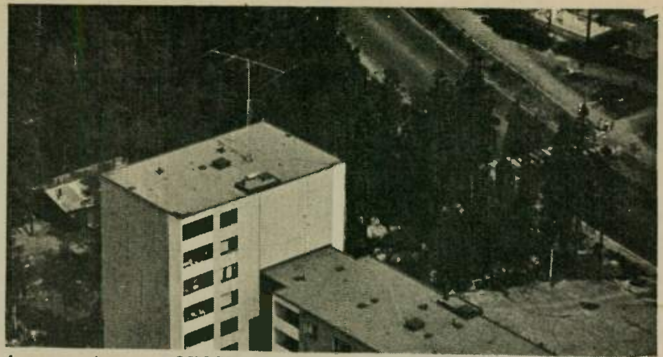
Antenna picture at OH2GH taken from airplane, The Hy-Gain 204BA at 150 feet off ground.
