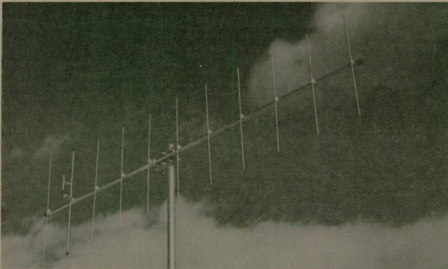
A147-11 The standard of comparison in VHF communication. Cut for FM and vertical polarization. Rated at 1000 watts with direct 52 ohm feed and PL-259 connectors. Boom 144", Longest element 40", Weight 6 lbs., Turning radius 72", Gain (reference 1/4 wave whip) 13.2 dB, Front to back ratio 28 dB, 1/2 Power beam 48 degrees, Wind area sq. ft. 1.21, Frequency MHz 146-148, Price $23.95. For 2-M DXers ask for the A144-11, cut for low end of the band, SWR @ Freq. 1 to 1, Price $23.95
