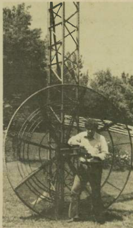
Jim Stitt, WA8ONQ, adjusts feed on 1296 MHz antenna.
