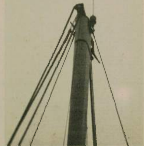
Marine VHF antenna used for 2 meters.
