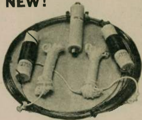
Heavy duty inductors with transparent tube covers.
