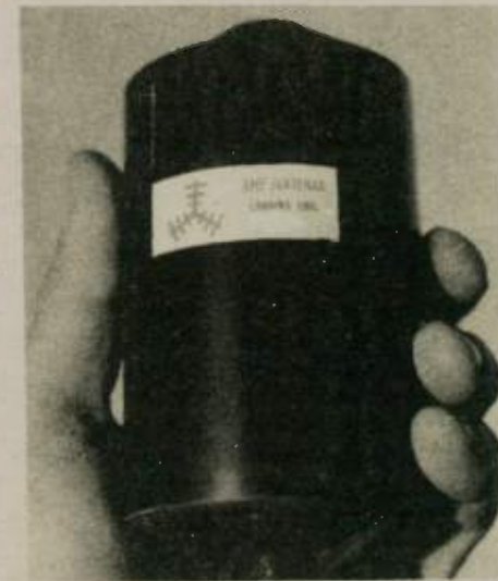
Loading coil for 160 meters. Be careful during coil changes!
