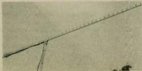
The 1296 MHz loop Yagi
