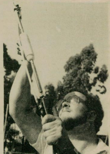
Coax feeding a backstay before sealant is added to top
