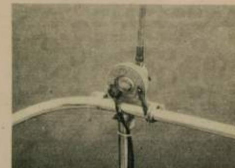
Rail-mounted whip. All coax connections are covered with Coax Seal.
