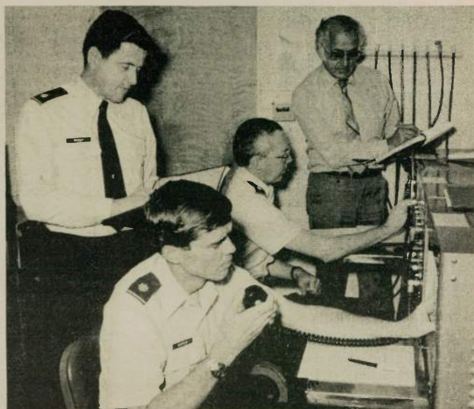
Shown operating two of the three HF radio positions are (left to right): Maj. Barry Priddy, K5VIP/AFA6CT; Maj. Ed Warren, K8RD/AFA6AZ (foreground); Lt. Col. Bill Stanfill, K4YCD/AFB6ME; and Paul Turkheimer, WA6NKL/AFA6YJ/AFF6P. The HF radios are Collins KW2A and 30L1 linears. Antennas include a Log Periodic, dipoles and "V" configurations.
