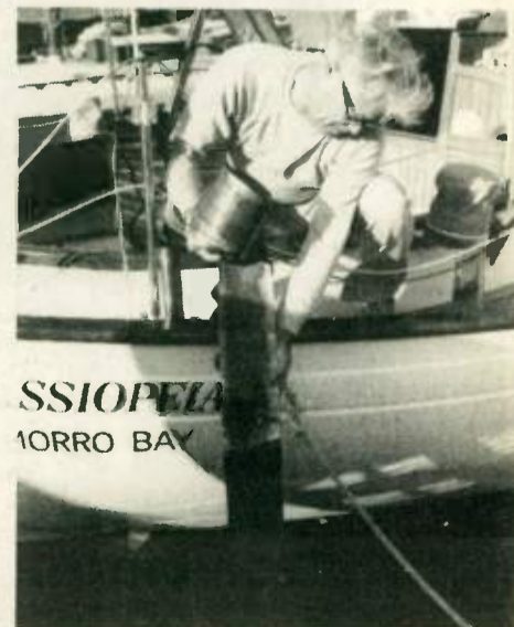
Testing for a foil/water ground
