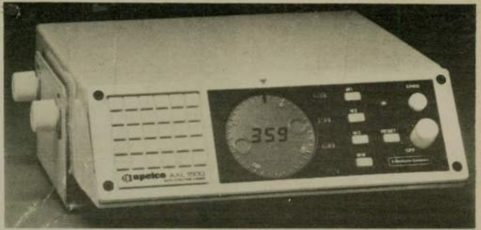
Apelco AXL 1500 Automatic Direction Finder that works with any VHF ham radio.
