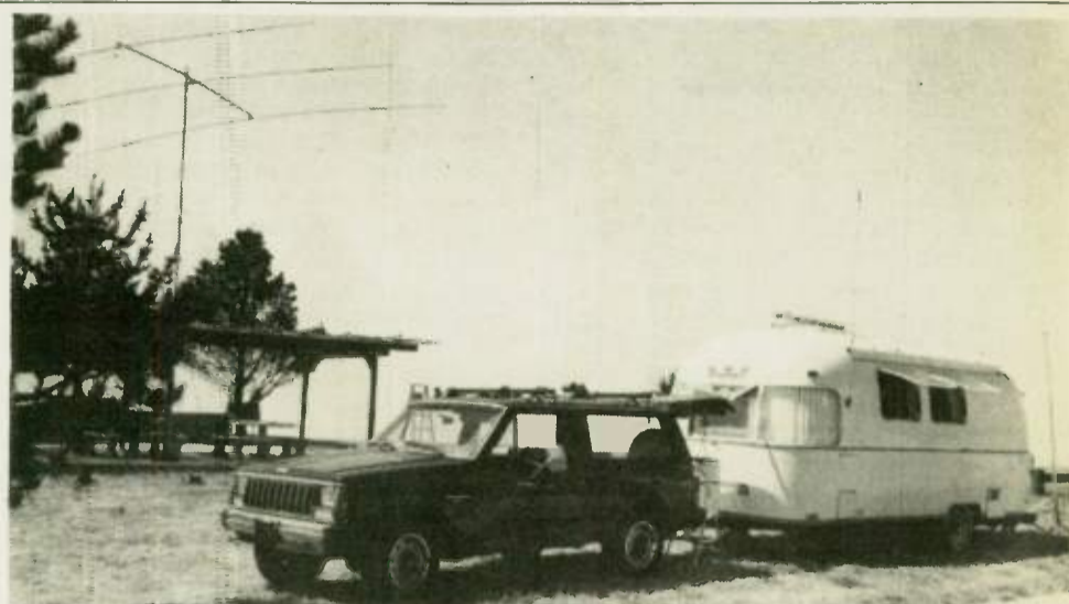
Overall view of the portable communications set-up with the temporary 3-element tri-band beam in place at San Pedro Hill AFS, Palos Verdes, California.
