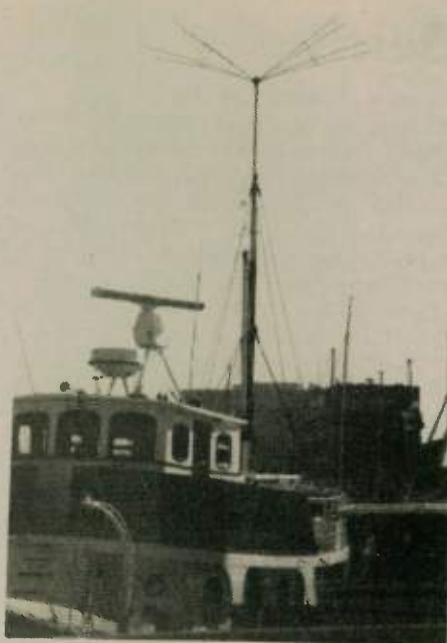
Mast-mounted dipole whips
