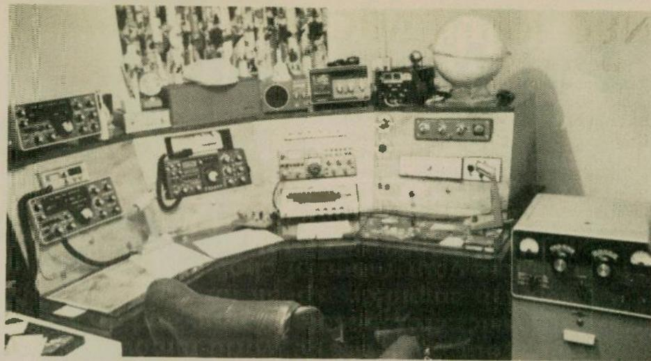
From left to right on top are: FR-101 receiver, 12-volt power supply, two speakers, SB-634 timer/wattmeter, and a 30-amp power supply. In the cabinet (left to right): FT-101 transmitter and Heath 20036-A 2-meter FM unit; FT-902 DM with rotator control on top; above MFJ keyboard is Kenwood
