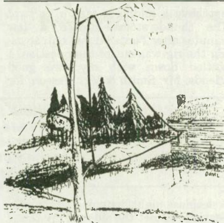
Figure 1 — W1FMR Loop between house and tree. Total length is 146', which is trimmed to resonance on 40M by grid dip oscillator or noise bridge. (Illustration courtesy of QRP Quarterly )
