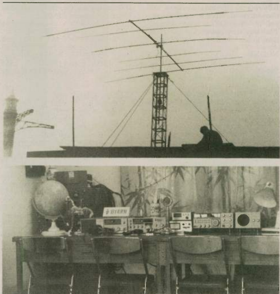
Gu, the operator of BY4RN, sends in these two photos. The station setup in the bottom was taken at the end of December 1987 with chairs for four operators. Notice the old D-104 microphone. The top photo shows the tri-bander used at the BY4RN in Nanjing. The antenna appears to be an old TH5DXX, the same type we have, which we have been using for about 18 years.
