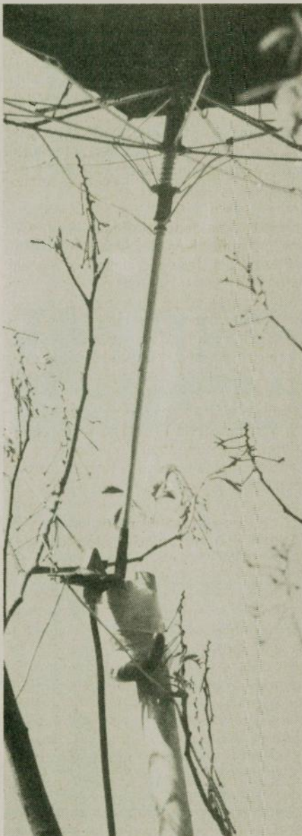
Budwig connector turns cheesy umbrella into an antenna.
