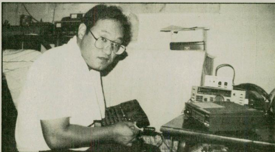
JA4RED testing the RTTY system used at N2HNO/KH8 in American Samoa. It consisted of a PK-232 with word processor and a FT747 Barefoot.
