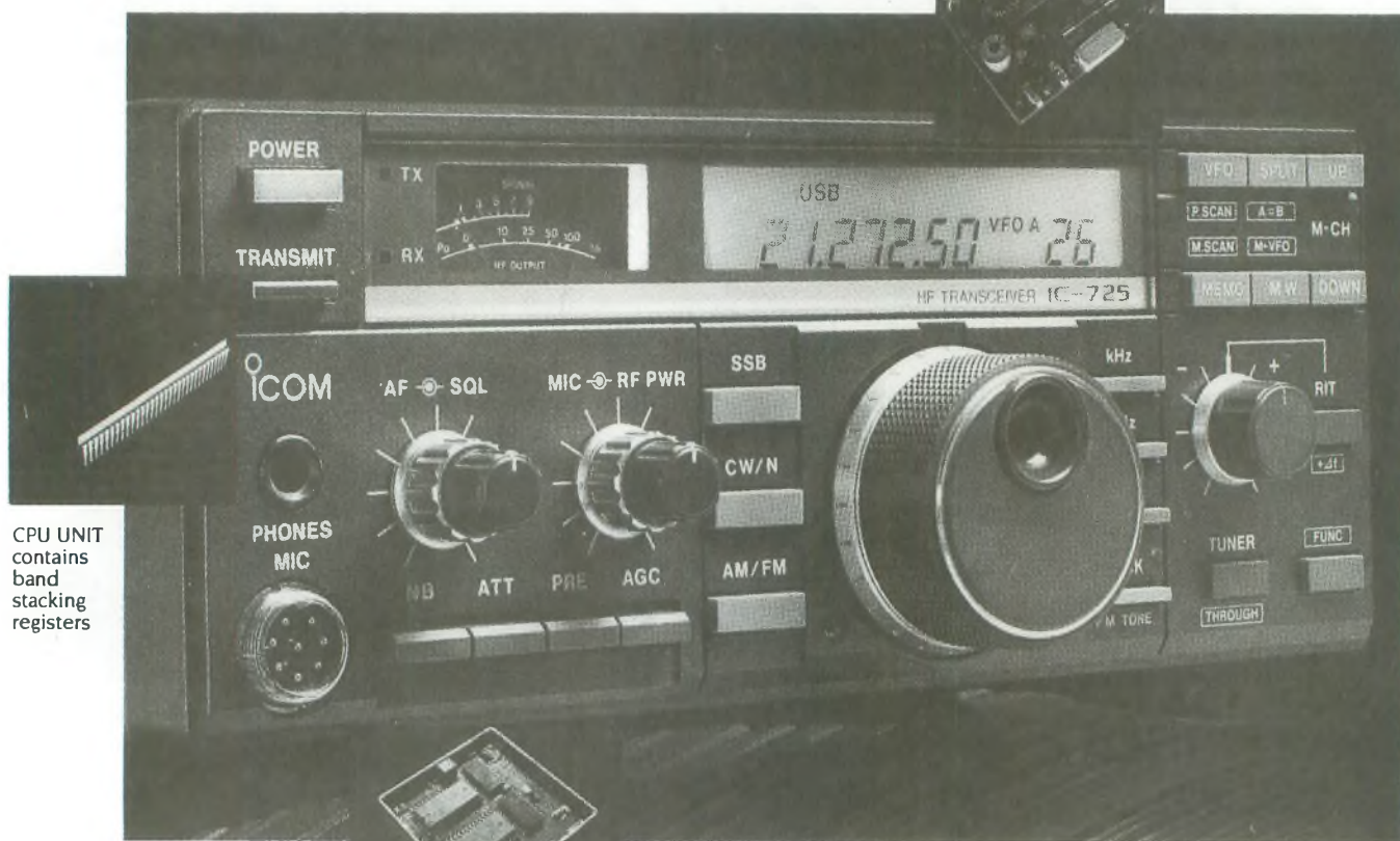
DDS UNIT provides excellent signal-to-noise ratio
