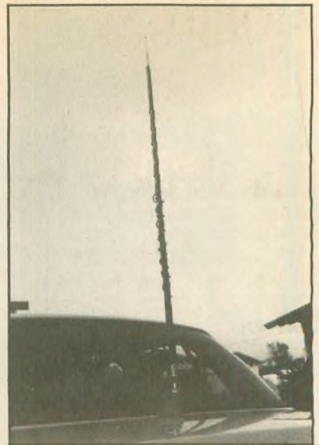
Trunk-lip Hustler mount: a perfect set-up for a no-holes installation, mounted up high.
