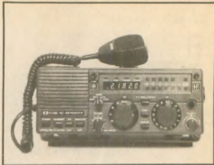
To get this marine ICOM to go to amateur lower sideband on 40 and 80M, just rotate the mode switch one click to the left of USB.
