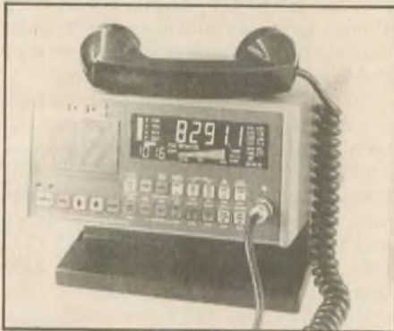
The new SGC2000 is specifically designed as an amateur and marine combination rig.
