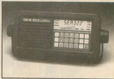
These marine Part 80 SSB radios all work well on amateur frequencies too.
