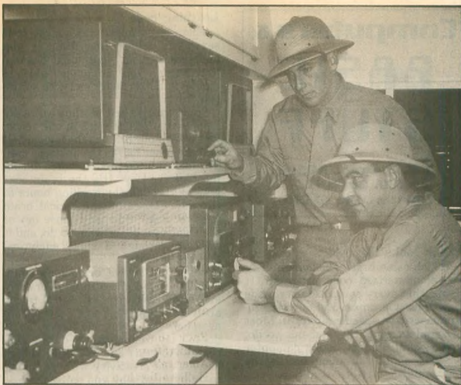
Interior of the Gatti-Hallicrafter's African Expedition ham shack trailer. Three Hallicrafters ham receivers are visible. Bob Leo, W7LR, now of Bozeman, Montana, has his hand on the Panadapter which scanned the band tuned by the receiver which Bill Snyder, W0LHS, is tuning. The picture was taken in New York prior to sailing for Africa, and the hats were the idea of an advertising agency genius.
