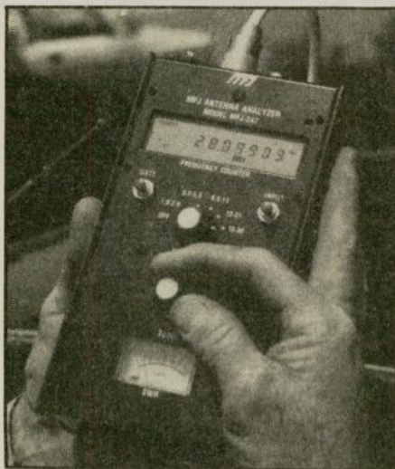
MFJ's SWR analyzer is easy to use to tune your HF whip.
