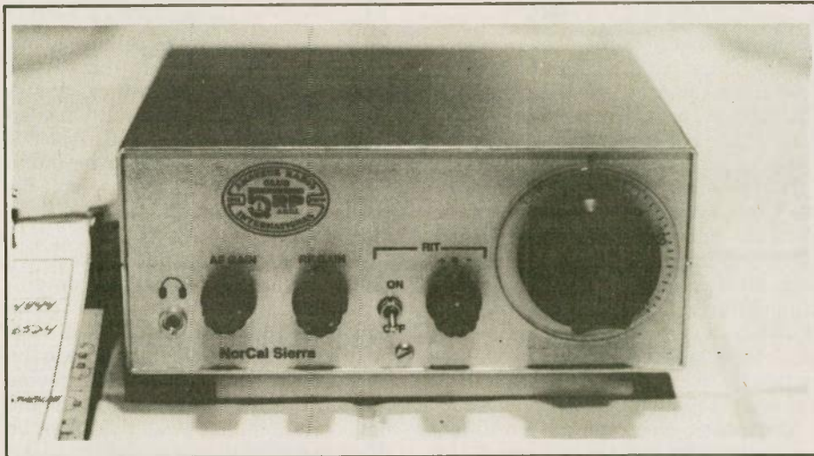
This prototype version of Northern California QRP Club's "Sierra" multiband QRP transceiver kit was used by Cam Hartford, N6GA, on a summer trip to Switzerland.
