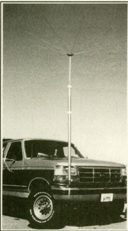
W6MMA prepared his capacity hat modified Broadbender BB3 for field strength testing. —photos by KO6AN
