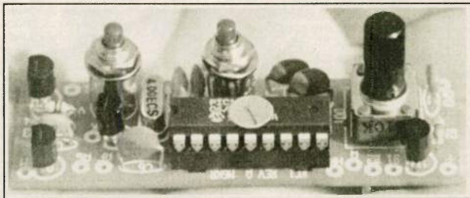
The Wilderness Radio KC-1 displayless frequency counter and electronic keyer. —photo by KI6SN
