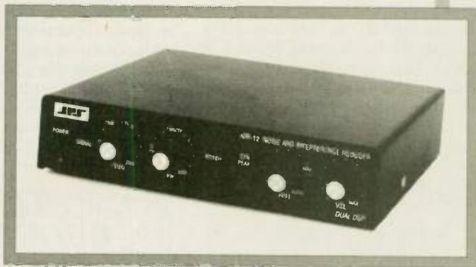
NIR-12 Dual DSP Noise Reduction Unit
