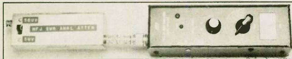
The attenuator and MFJ SWR analyzer interconnection. —photos by KZ6O
