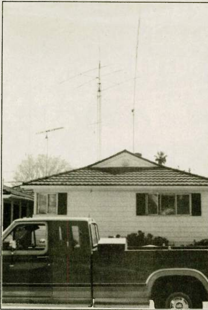
A 45' tower with a Cushcraft A3, and an R7 up in the air. —photos by N6WR
