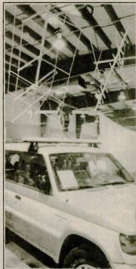
Montero equipped with az-el rotator for satellite links, built by Woodhouse Communication.
