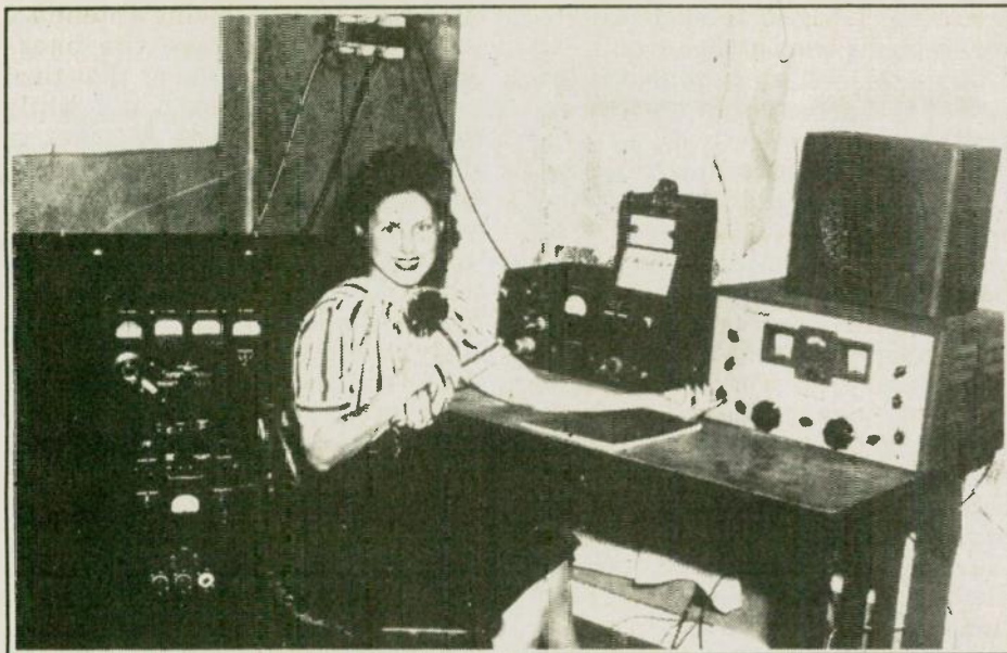
The Texas Dewdrop, Mary Palmer, W5DEW, in 1946. From left to right: A HT-4 Hallicrafters transmitter (actually it is an army surplus Signal Corps BC-610 that her then husband, Buz Palmer, W5BUZ, bought after World War II ended), The Dewdrop, transmitter control panel, and a HQ-129 Hammarlund receiver.
