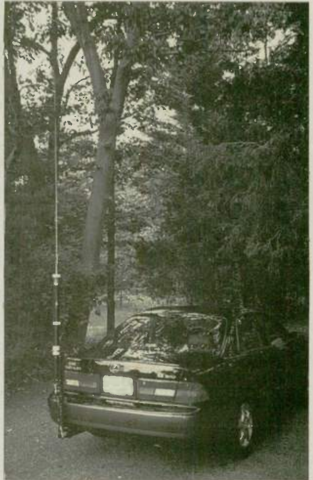
Left: Joel's mobile installation looks factory installed. Above: The screwdriver antenna is mounted on a left rear frame.
