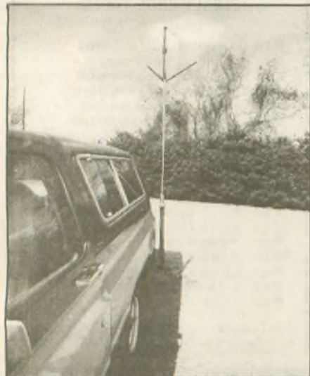
The Spider offers 4-band auto-tune without having to stop and change bands.
