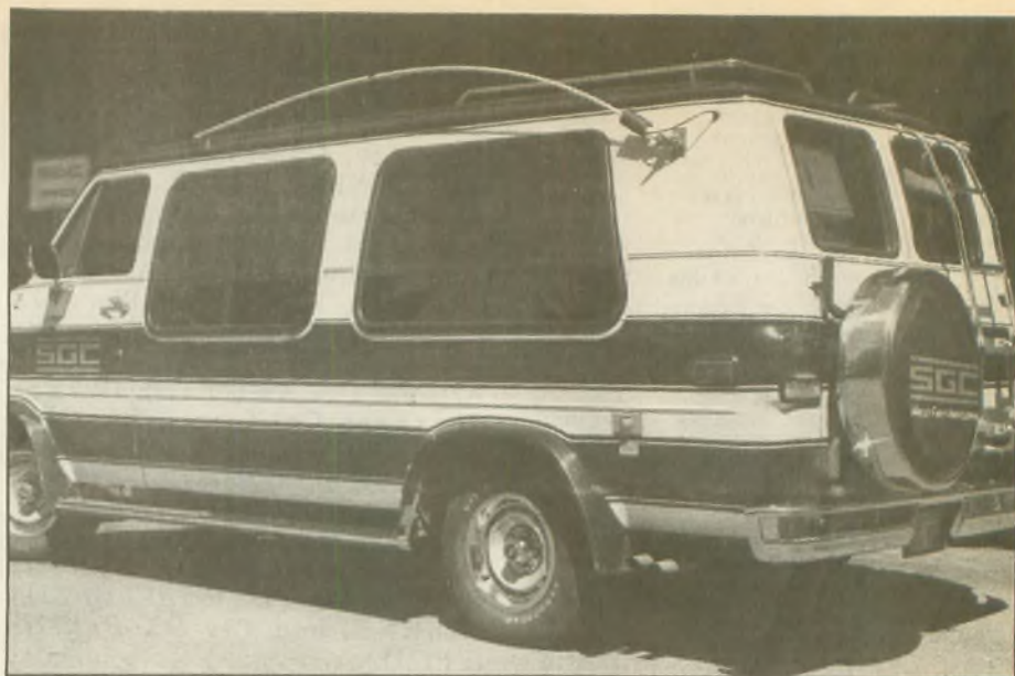
The SGC Model 303 HF whip installed on a van (tuner inside the vehicle).
