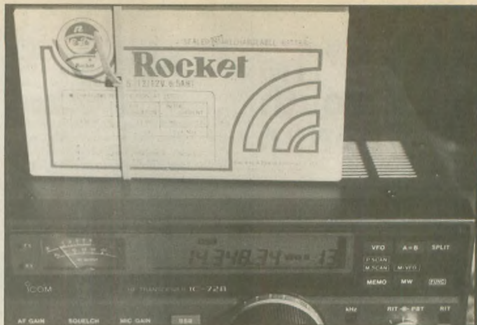
Temporary Icom mobile installation with sealed rechargeable battery.
