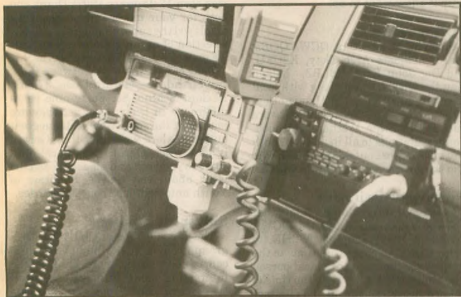
A neat dual-radio mobile installation featuring two remote heads.
