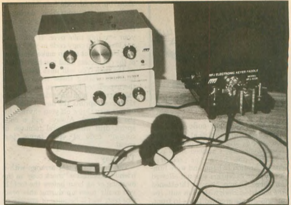
Here's a look at the tidy QRP setup of Bob Schnick, KA3YJG. That's an MFJ 9030 transceiver sitting atop an MFJ 971 tuner.
